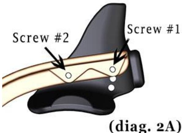
**Upon completion of steps 1-2**, once you are 100% happy with the fit of your restraint, we recommend that at this time you remove all screws one at a time (except screw #2 in step 2) and secure them with tread lock “blue” and tighten snug.
